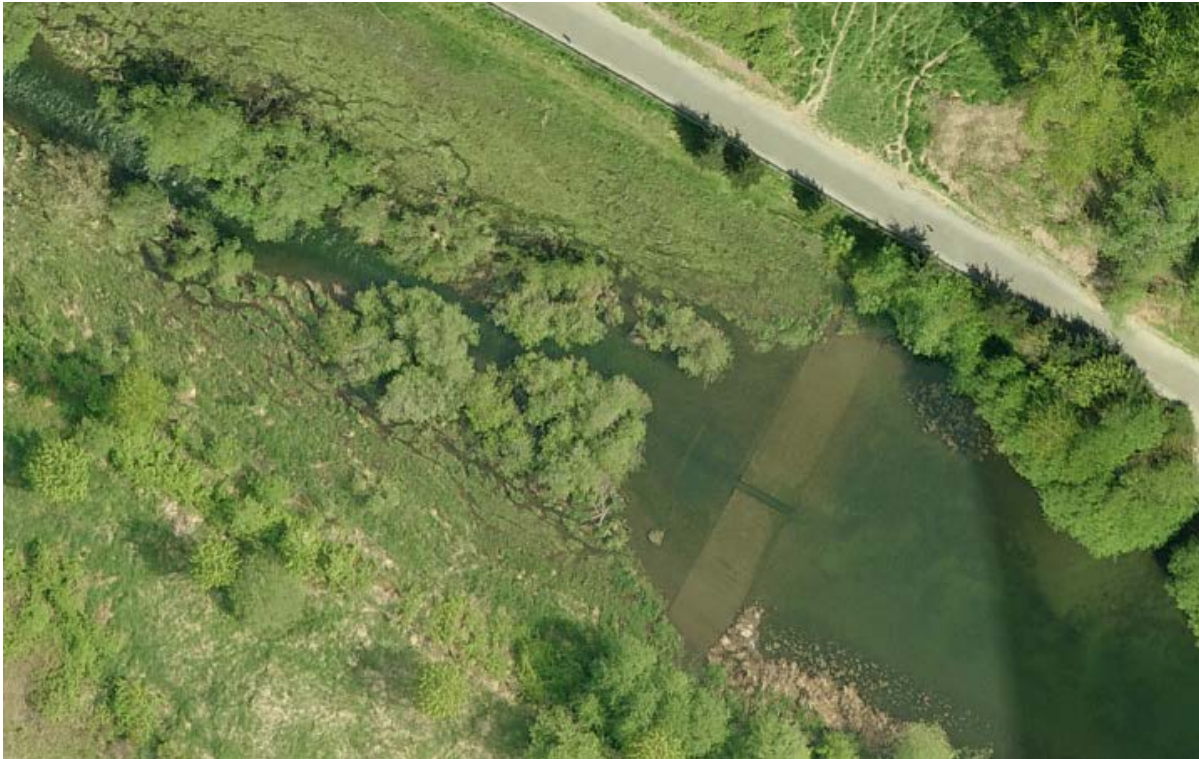
Figure 4. Weir (showing low-flow notch) as well as channels through willows and reed canarygrass (2009 aerial imagery).
